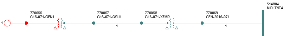
Figure 0-2: GEN-2016-071 Single Line Diagram (Modification Configuration)
